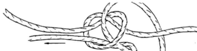
Figure 7 The end of the rope is then looped over the rope that was fed through the first overhand knot to make the second overhand knot. Feed the end of the rope our through the center of the first knot, passing on the same side of the loops the rope leaving the original knot
