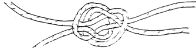
Figure 8. Align the two overhand knots under each other and tighten. Make adjustments, if necessary, to ensure the correct spacing for the halter.
