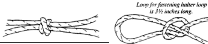
Figure 9. The final knot should look like this Even though flit, overhand knots might he properly tied, you might need to rearrange the knot to form properly when tightened
